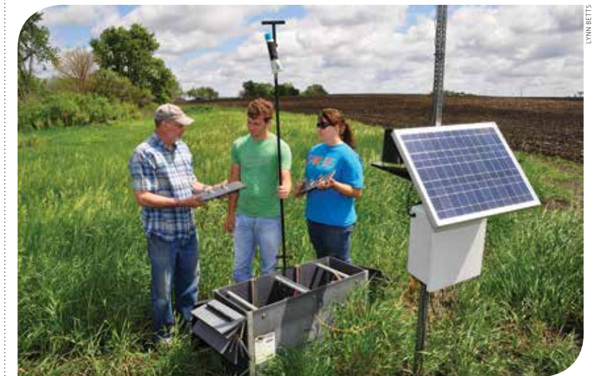
Conservationist Bruce Voigts explains how stop logs slide down into a water control structure to control water levels in a saturated buffer in north central Iowa. Solar powered measuring equipment documents water flow and weather conditions.
